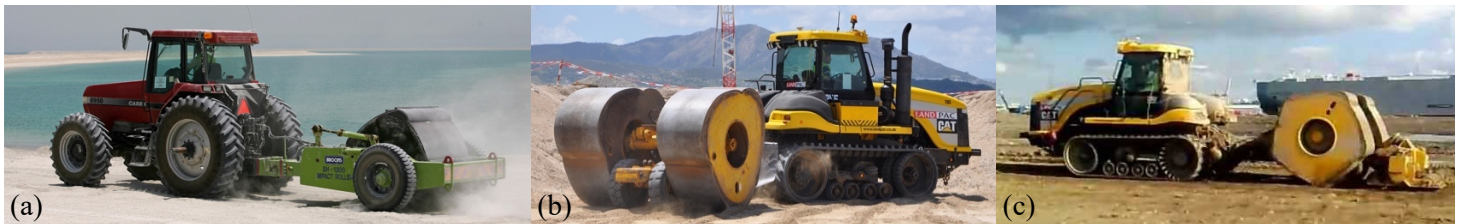
Fig. 1: Rolling dynamic compaction modules: (a) 4-sided (Broons); (b) 3-sided (Landpac); (c) 5-sided (Landpac).
